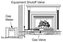
Figure 35 - Checking Gas Joints for Natural Gas Fireplace
